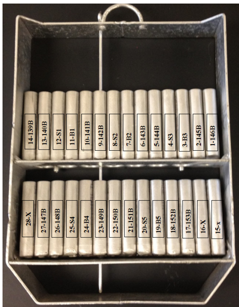
FIGURE 2: The sample holder with the hinges closed. The first number represents the position number (1-28) in the sample holder. The second number is the sample (139B-153B), the plastic clay standard (S1-S5) or brick clay quality control (B1-B5). The sample holder faces the reactor core from this position.
