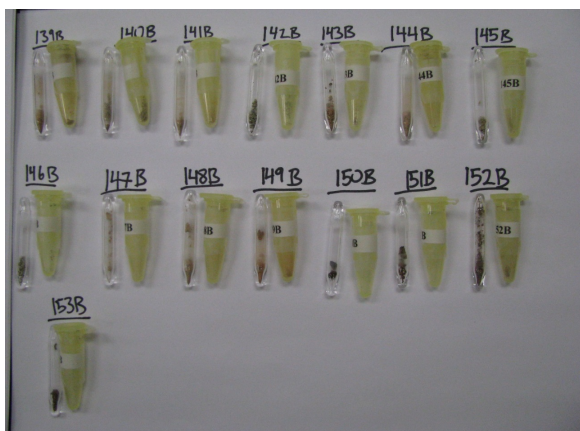
FIGURE 3: Fifteen Italian tile samples after being sealed in quartz ampoules.
